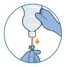
Pull the water feed spike out of the water reservoir.
