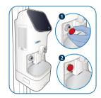
Cover the gas outlet adapter with the protective cap.
