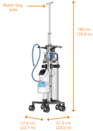
Figure 9-2. HAMILTON-HF90 with trolley dimensions
